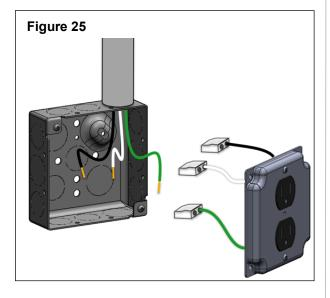
6. Match the wire colors, then grip the wire firmly and push the conductor into open port of the push in connector (Figure 26).
