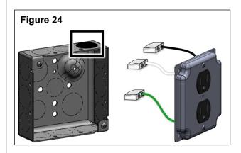
Install conduit into the knockout opening and pull the green, white and black wires into the box. 5. Strip the green, white, and black field supplied wires 1/2 in. Make sure the conductors are completely bare (Figure 25).
