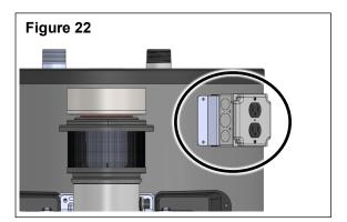
2. Remove the two screws around the outlet cover. Remove the outlet cover and prewired outlet (Figure 23).
