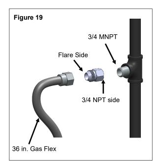
3. Thread the flare side of the 36 in. Gas Flex into the flare side of the Gas Flare Adapter (Figure 20).
